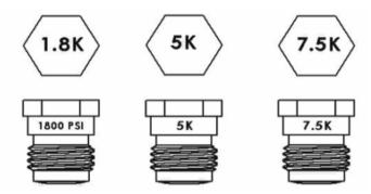
WARNING: IT IS ABSOLUTELY ESSENTIAL THAT YOU ONLY REPLACE FAILED UNITS WITH EXACT REPLACEMENTS. ASTM UNIFIED BURST DISKS HAVE THE PRESSURE IDENTIFICATION STAMPED ON THE HEAD OF THE DISK. SOME DISKS MAY HAVE THE PRESSURE IDENTIFIER ON THE SIDE OF THE DISK. SEE ILLUSTRATION. WARNING SERIOUS INJURY OR DEATH MAY RESULT FROM IMPROPER BURST DISK SELECTION AND INSTALLATION.
